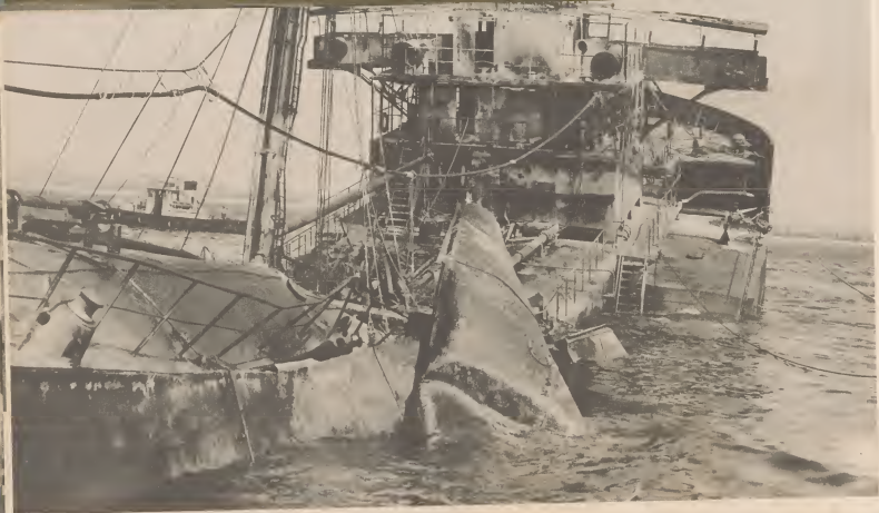
Smashed and burned by a German torpedo that struck it just off Aruba's shoreline, this ship, the Pedernales , sailed again. Divers cut it in two pieces, and the separate sections were
